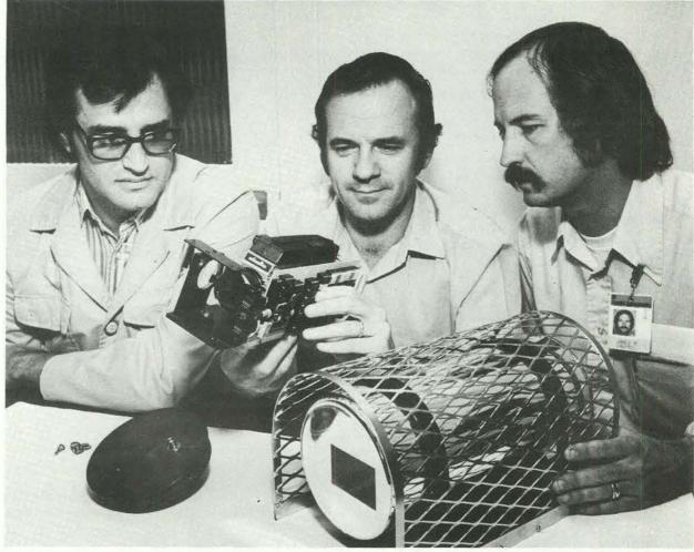
NEW SURVEILLANCE CAMERA is displayed by John Aragon (1754), Dick Striker (9622) and Jim Campbell (1754). The tamper-proof unit is designed to monitor nuclear generating plants or nuclear fuel processing and storage areas.
